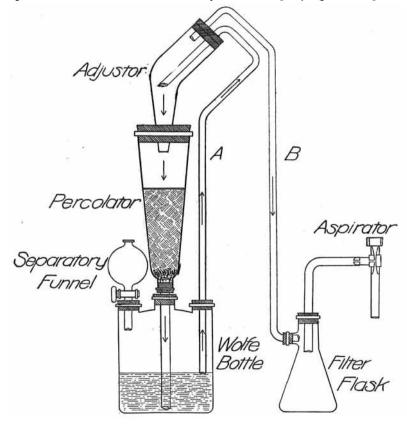
is adjusted to such a height in the menstruum in the Wolfe bottle that, when emptied by suction, it will transfer a convenient amount of the liquid to the drug in the percolator. The arrows point the direction of flow. When A is emptied, there is a difference of pressure in the system equal approximately to the weight of the liquid transferred to the percolator. This liquid then percolates through drug to
